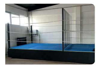
FAYSIM offers real life experience in a risk-free environment with earthquake scenarios. Users must achieve task in 3 different stages. (Before, during and after the earthquake) The shaking platform of the simulator works synchronously with the virtual reality application, and it gives a real earthquake feeling. Users can explore the virtual rooms only by the walking literally on the vibration platform. Earthquake simulation works with hand tracking, without any need of control device.
